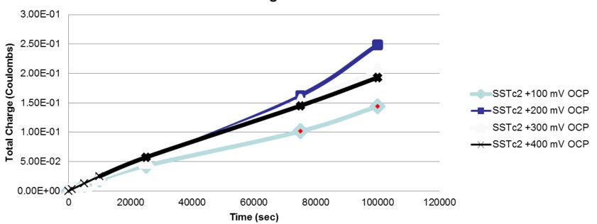
SSTc2 Charge Plot vs Potential
