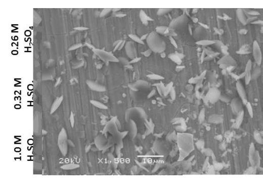
Figure X. Insert Tc electrodeposition images from solution on Cu.....
