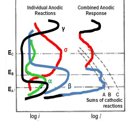
The Stern-Geary equation predicts that for  $E > E_{CORR}$  the anodic reaction predominates and for  $E < E_{CORR}$  the cathodic reaction predominates.
