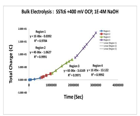
Assuming uniform release of Tc, total mols ~ 2.529E-9 Tc release rate: 3.025E-12 mols per hr Time = 3,010,000 sec Tc Current: 1.25E-16 Amps Compare Tc metal ~ 1-2 orders of magnitude greater release from bare metal
