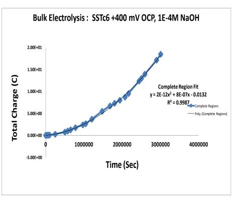
Assuming uniform release of Tc, total mols ~ 2.529E-9 Tc release rate: 3.025E-12 mols per hr Time = 3,010,000 sec Tc Current: 1.25E-16 Amps Compare Tc metal ~ 1-2 orders of magnitude greater release from bare metal
