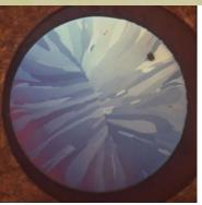
Microscopic cross section of irradiated Tc target Konings et al., http://www.nea.fr/html/pt/docs
